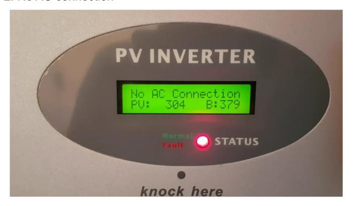
Meaning: inverter detects no AC voltage from the AC side.
